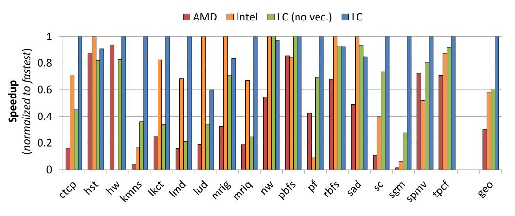
LC (with vec.) outperforms AMD (without vec.) and Intel (with vec.) by 3.32x and 1.71x
